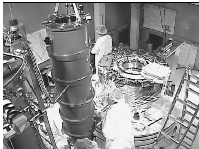
Fig 5: Assembly of the CDMS apparatus in the Soudan mine during 2002. The system is now fully operational and is starting to take data.
